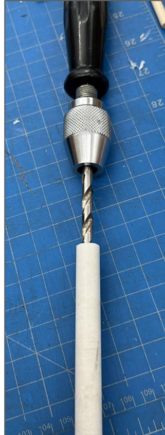
3D printed pipe but it's too small! I realise I should have done test prints beforehand to make sure that the hole was large enough and I accounted for the filament width.
