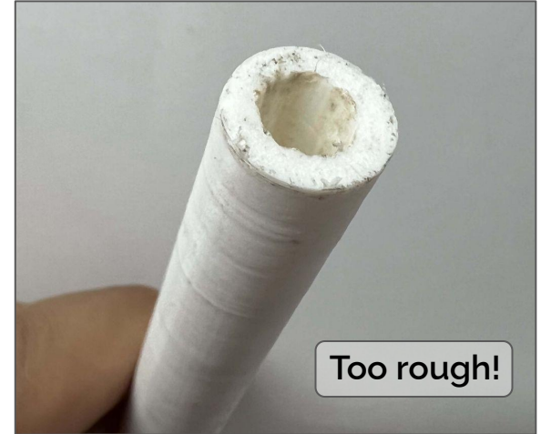
I used two main methods to try and fix this for the prototype. Firstly, I tried widening it by twisting a 0.25" handscrew through the hole but that did not work. Then I fed the hot wire foam cutter wire through the hole and tried to burn off the inside edges but that made the hole too rough and no candies could fit. I had to reprint!
