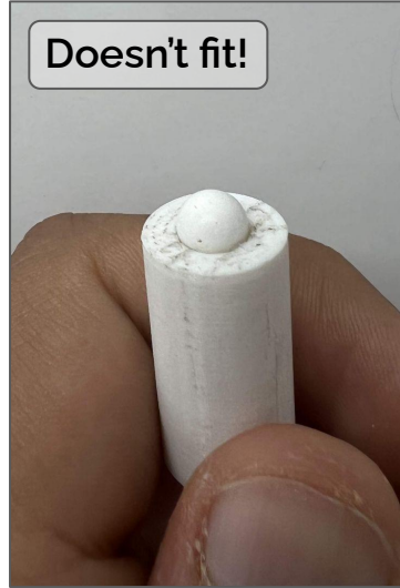
3D printed pipe but it's too small! I realise I should have done test prints beforehand to make sure that the hole was large enough and I accounted for the filament width.
